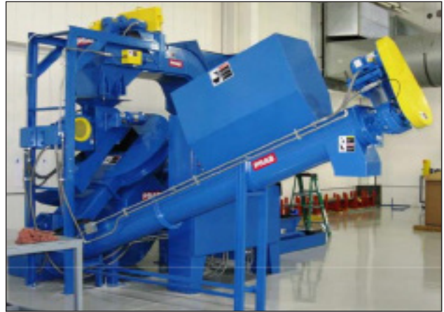
PRAB 24CD Wringer System (chips discharged to screw conveyor)
