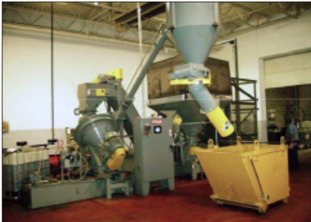
PRAB 24AD Wringer System (chips discharged to scrap cart)
