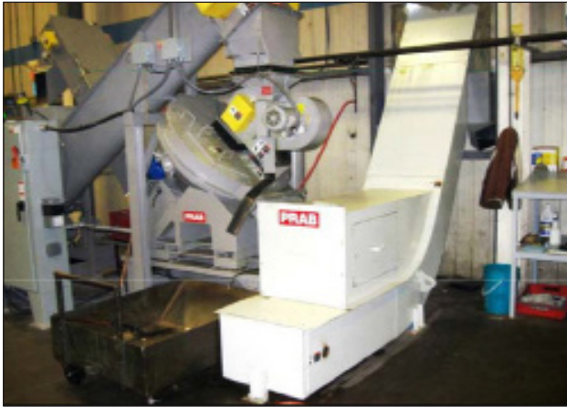
PRAB 24CD Wringer System (chips discharged to outdoor silo)
