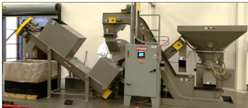
PRAB 24CD Crusher/Wringer System (chips discharged to screw conveyor)
